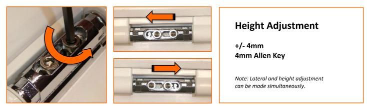
Slacken off both M5 Cap Head Screws **on all hinges** (and ensure they are retightened after adjustment). The door can now be moved up or down about the nominal position.
