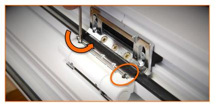
Open the door to expose the Compression Adjustment Grub Screws. Rotate the Grub Screws counterclockwise to increase compression.
